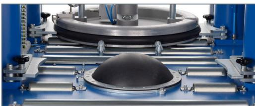
Optional pneumatic drum support. Helps to save additional 50% of residual material.
