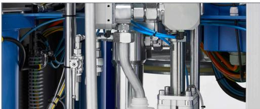
Optional **airtract** pump de-aeration system with material recirculation allows up to 90% material savings compared to manual venting.
