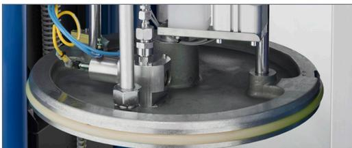
Automatic aeration system for fast, safe and clean drum exchange.
