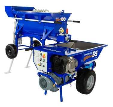
from 0 to 20 bar Product pressure Product flow-rate from 0 to 55 kg/min Machine motor power 5,5 kW 366 L/min Comp. absorbed air flow-rate Compressor power 2,2 kW 400 V - 16 A - 50 Hz Power supply 100 L Machine tank capacity 6 mm Maximum grain size Integrated vibrator ves Pump **MAP 11** Mixer motor 2,2 kW Mixer tank capacity 100 I 115 x 65 x 73 cm Machine dim. (L x w x h) 129 x 74 x 126 cm Mixer dim. (L x w x h) Machine weight 160 kg Mixer weight 107 kg Noise level 96 Lwa
