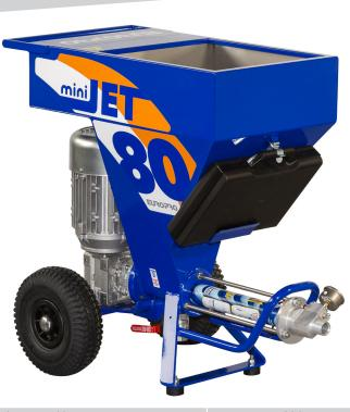
Maximum working pressure 80 bar Maximum product flow-rate 4,5 L/min Electric motor 1,5 kW 230 V / 50 and 60 Hz Power Type of pump volumetric screw Pump JET 1 45 L Tank capacity 0.045" Maximum nozzle size (new) 66 x 43 x 71 cm Dimensions (L x w x h) Weight 53 kg Noise level 91 Lwa
