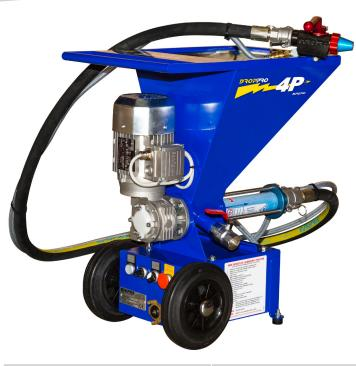
Product flow-rate 0 to 4 kg/min 0,55 kW Motor power Electrical supply 230 V 50 and 60 Hz Frequency 3,64 A Motor current 20 L Tank capacity 1,5 mm Maximum grain size 30 bar Maximum pressure 10 bar Minimum pressure Pump MAP 3 Air coupling express Dimensions (L x w x h) 66 x 43 x 71 cm Weight 35 kg
