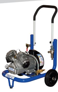
Rotation speed 2850 RPM Flow-rate of air absorbed 366 L/min (22 m<sup>3</sup>/h) Quantity of oil (crankcase) 0,44 L Oil consumption 1,4 q/h Motor power 2,2 kW Electrical supply 230 V 50 Hz Frequency Current 13 A Thermal protection yes Safety valve yes Tank capacity 1,52 L Maximum pressure 10 bar quick-connect Air coupling Dimensions (L x w x h) 59 x 55 x 86 cm Weight 36 kg Noise level 92 Lwa
