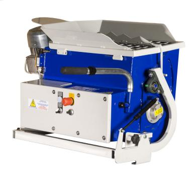
CP Joint 20, Machine compatible with CP 30, 35, 40, 45 & 55 Mixing type sequential 1,1 kW Motor 28 to 80 RPM Forward / reverse rotation speed 230 V - 10 A - 50 & 60 Hz Power supply Tank capacity 70 L Water meter no Mixing paddle blades Loading height 135 cm Dimensions (L x w x h) 88 x 52 x 57 cm Weight 75 kg
