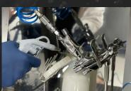
Connect the compressed air coupling to the air 2 connection of the spray gun.
