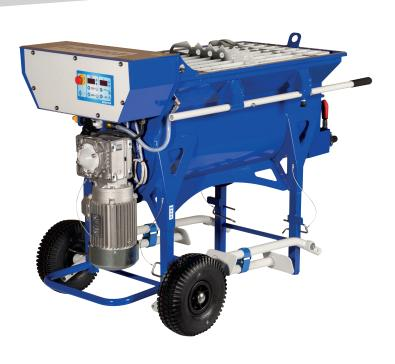
Décopro Joint, CP 10, 15, 20, 25, Machine compatible with 30, 35, 40, 45 & 50 Mixing type sequential Motor 2,2 kW 36 to 84 RPM Forward / reverse rotation speed 230 V - 10 A - 50 & 60 Hz Power supply 100 L Tank capacity Water meter integrated Mixing paddle double helical paddle Loading height 126 cm Dimensions (L x w x h) 129 x 74 x 84 cm Dim. high position (L x w x h) 129 x 74 x 126 cm Weight 107 ka
