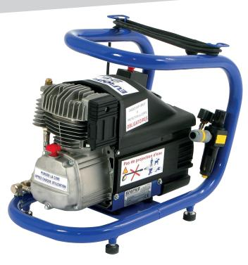
2850 RPM Rotation speed Flow-rate of air absorbed 235 L/min (14 m<sup>3</sup>/h) Quantity of oil (crankcase) 0,35 L 0,5 q/h Oil consumption Motor power 1,8 kW Electrical supply 230 V 50 Hz Frequency 10 A Current Thermal protection yes Safety valve yes Tank capacity 2 L Maximum pressure 10 bar quick-connect Air coupling Dimensions (L x w x h) 58 x 34 x 55 cm Weight 24 kg Noise level 92 Lwa
