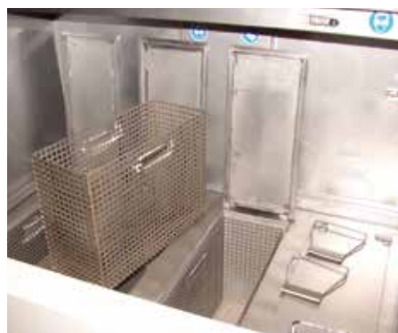
▲ Paint stripping tanks with baskets
