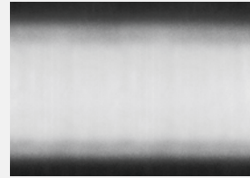
Latex emulsion paint through a HEA 517 tip at 70 bar
