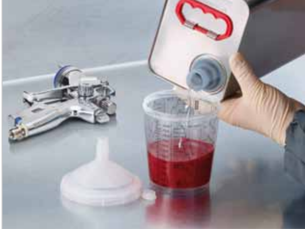
The paint is mixed in the cup later used for painting.
