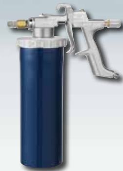
■ SATA® HRS™ E Pressurised cup spray gun with 1.5 l cup, for cavity preservation and underbody protection applied out of disposable containers, with material flow control, hook and nylon wand and round fan nozzle. Art. No. 172882
