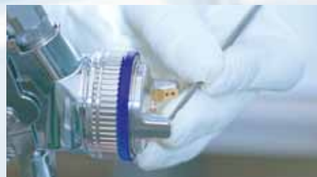
Hand adjustment: Each nozzle set is separately manually "tuned" to optimise the spray fan.
