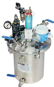
MDG 8 KLA with air-driven type 46-810 agitator, capacitive fill level sensor as well as bottom valve for filling and two additional upper valves for material recirculation.
