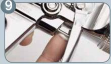
Grease visible part of air piston rod
