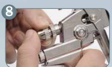
Install material flow control screw
