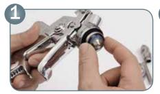
Assembly of the fluid tip
