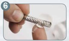
Grease and insert paint needle spring
