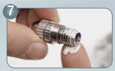
Grease thread of material flow control screw
