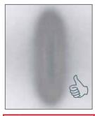
Dirt or damage, especially on nozzle set components, can provoke faulty spray patterns. In most cases, dirt can be removed easily.
